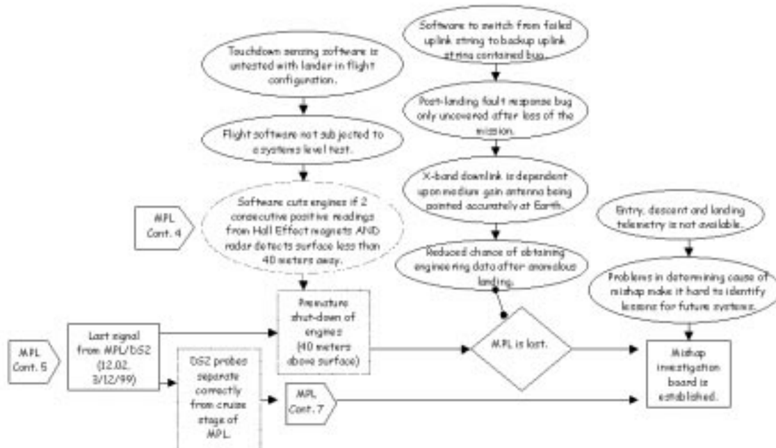
Figure 10.24: An ECF chart of the Polar Lander Mission Failure
