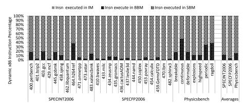
Fig. 4. Dynamic x86 instruction distribution in IM, BBM and SBM
