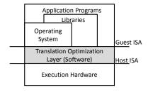
Fig. 1. HW/SW interface in co-designed processors
