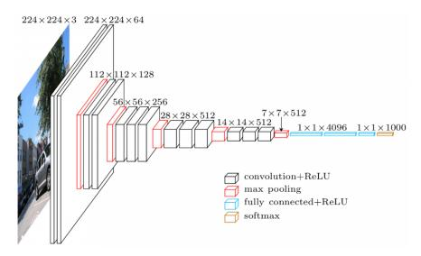
Fig. 1: VGG-16 neural network architecture.
