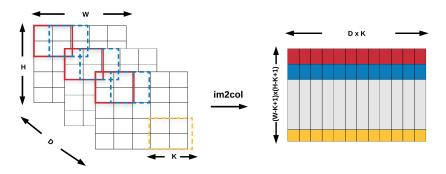
Fig. 5: Im2Col operation in input matrices.
