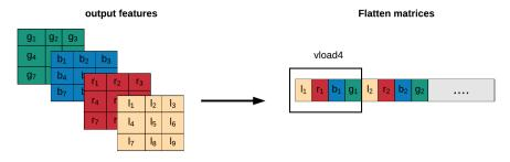
Fig. 4: Flatten matrices by depth.
