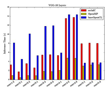
Fig. 3: Time for Serial C, OpenMP, and baseline OpenCL implementations.
