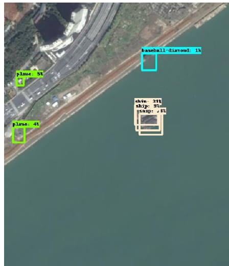
Figure 10: Instances Detected in Image P2310 after Running it through Model SSD. Each Instance has a Bounding Box with the Associated Class and Confidence Score
