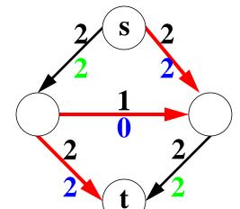
Send another unit of flow through the network. Note that there still exists an augmenting path, that can proceed *backward* against the directed central edge.
