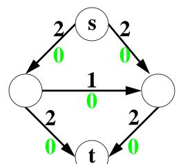
Initialize the network with a null flow. Note the **capacities above the edges**, and the flow below the edges.
