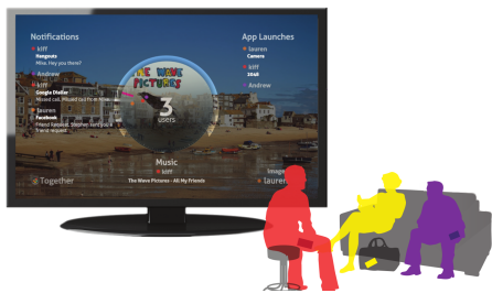
Figure 6: Cast Together is a situated display (SD) prototype designed to support multiple smartphone users in an intimate co-located situation, who can negotiate interruptions on a shared display without removing the smartphone from a bag or pocket.
