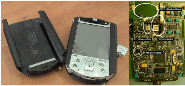
Figure 1: Left: Mesh device alone and attached to an HP5550 Pocket Pc. Right: The MESH circuit board showing the main components related to the navigation task
