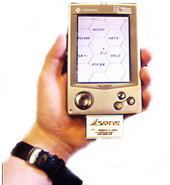
FIGURE V.14: PocketPC augmented with XSens miniature linear accelerometer.
