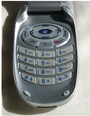
FIGURE V.13: Keypad text entry. Letters are coded as sequences of digits. In the T9 system, each letter is coded as a single digit, and the entire word decoded at the end.
