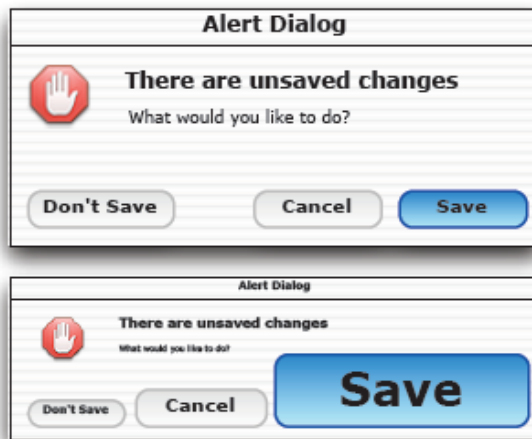
FIGURE V.2: The visual space (a) and motor space image (b) of a dialog box with variable control-display ratios. The “save” button, which has higher utility to the user, is enlarged in motor space. From Blanch et al. [2004].
