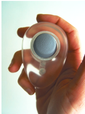
FIGURE V.8: SonicText. The joystick can move in eight directions; each letter requires either a single directional movement, or a directional movement followed by a “roll”. Audio feedback is presented during the interaction to reduce the need for visual attention. From Rinott [2004].
