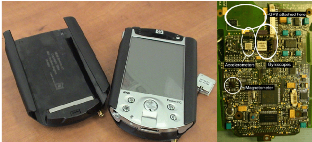
FIGURE IV.15: PocketPC augmented with GPS sensor pack. The sensor pack include GPS, 3-axis accelerometers, 3-axis gyroscopes, 3-axis magnetometers, capacitive touch sensing and vibrotactile display
