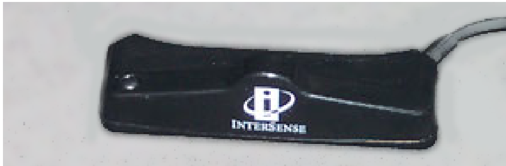
FIGURE IV.7: InterTrax head tracker used for the manipulation of the time horizon in the rolling object demo. Tilting up and down extends and retracts the prediction horizon.
