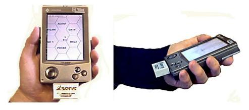
Fig. 4. The system running on Cassiopeia E115 with a miniature accelerometer
