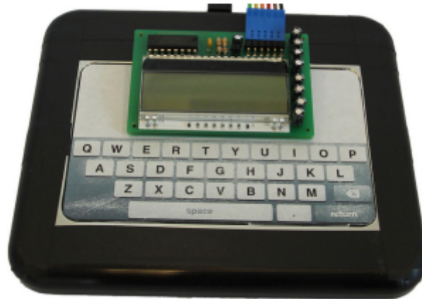
Figure 2.7: Figure showing the prototype built for the ForceType implementation [27]
