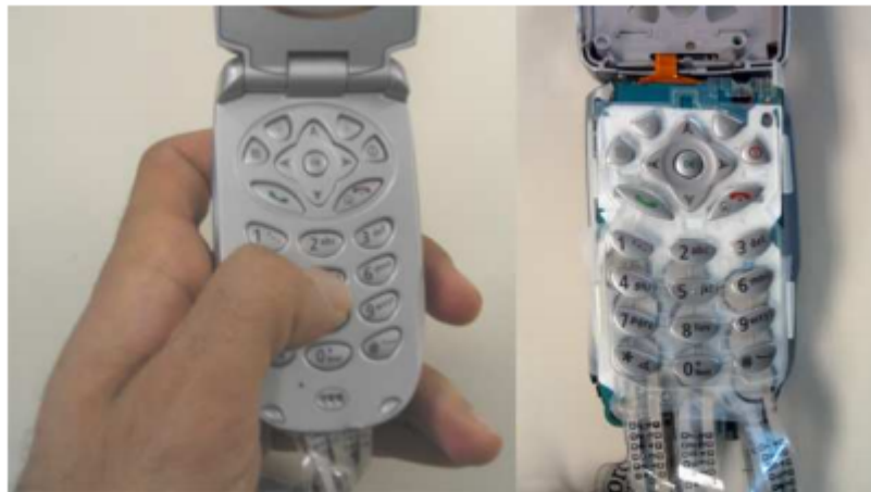
Figure 2.3: Figure illustrating how capacitive sensors were inserted under the buttons [7]
