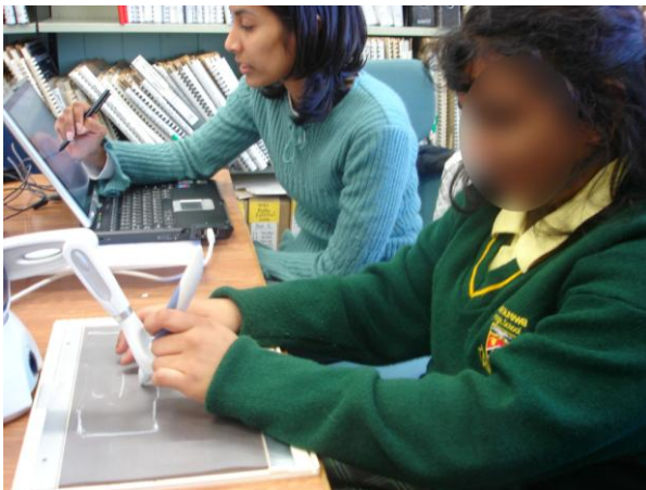
Figure 3: The McSig system in use. The teacher (on the left) draws on a Tablet PC to create a shape and the student (on the right) can feel, explore and be moved around the shape.
