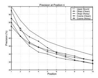
Fig. 5. This plot shows the Precision as a function of the ranking position. The results are obtained by averaging over all queries.
