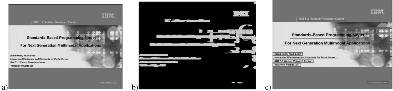
Fig. 3. Text line detection process. (a) Original image. (b) Potential text pixels. (c) Candidate text lines.
