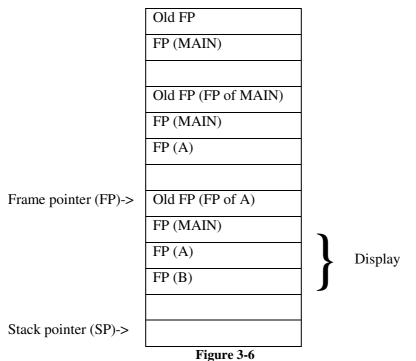
Similar to MAIN calling A, when B is called from A, it saves the old frame pointer – which is now the frame pointer for A – to the stack, but this time copies two frame pointers from the display A created. As with the other cases, it then copies its own frame pointer to the end of the display, and moves the frame pointer to point to the top of its stack frame.
