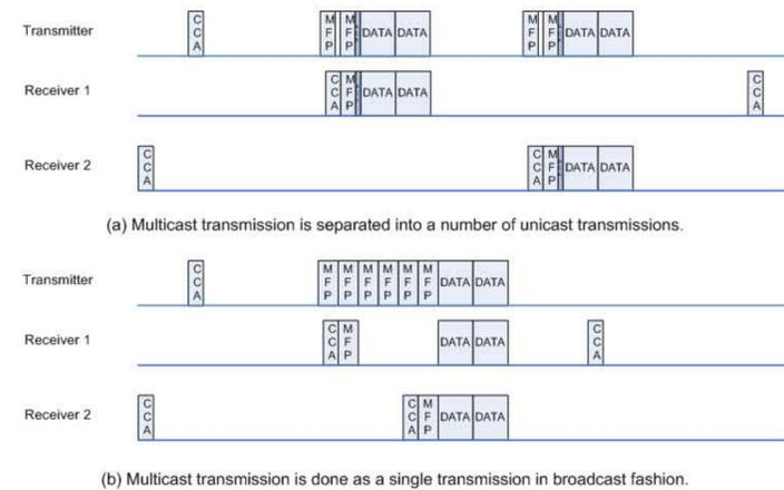
Figure 3. Operational cycle in the case of multicast transmission.
