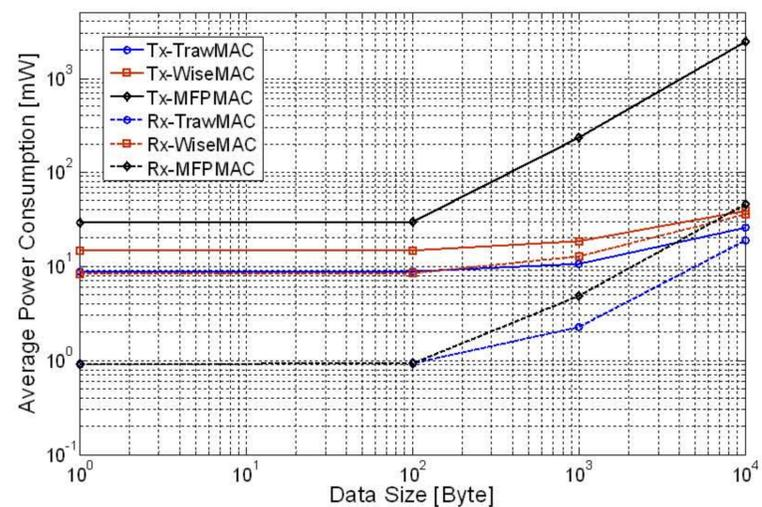
Average power consumption of TelosB running TrawMAC, WiseMAC and MFP-MAC for *unicast* transmission. TrawMAC reduces the energy consumption on data transmission significantly regardless of the transmitted data size while providing improvement on the reception side at burst data reception.
