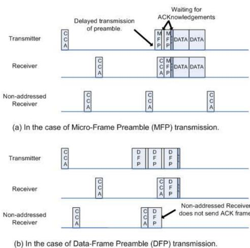
Figure 2. Operational cycle in the case of unicast transmission.
