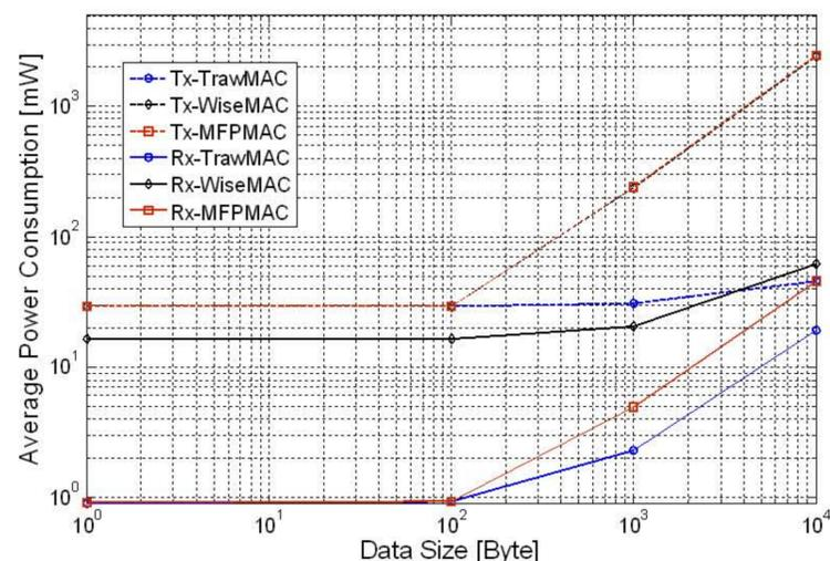
Average power consumption of TelosB running TrawMAC, WiseMAC and MFP-MAC in *broadcast* transmission. TrawMAC shows minor energy efficiency improvement over small data sizes which becomes significantly large in case of bursty traffic.
