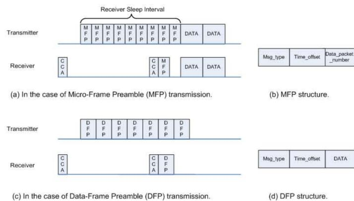
Figure 1. Operational cycle in the case of broadcast transmission.
