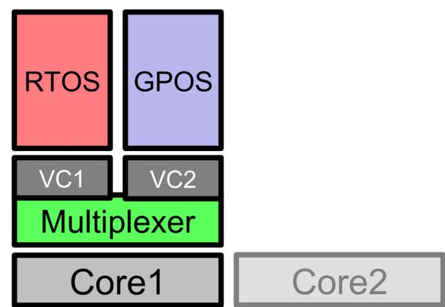
Fig.5 Stopping a core to save power consumption
