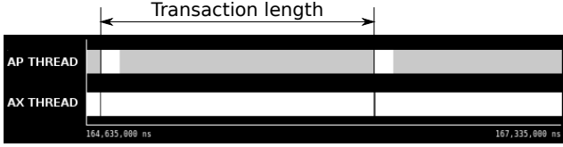
(b) Spin-only: Static allocation of extra resources to auxiliary threads at commit phase.
