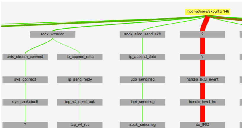
(b) A multi-backtrace (mbt) query for a specified line of code reveals the many contexts in which it was encountered. Note that the full graph is much larger than what we can reproduce in this paper.
