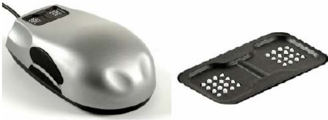
Figure 1. The VT Player Mouse (left) and a close up of its two pin array cells (right).
