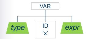
put the identifier 'x' into the type table, along with the type.
