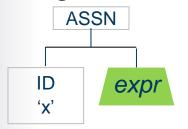
lookup 'x' and retrieve its type; walk *expr* and note its type; check that the two types are equivalent
