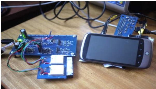
Figure 1: Nexus One phone, FSR's and microcontroller are attached to the back of the device. On the left is the Peltier Microcontroller with two Peltier heat pumps detached from the back of the phone.
