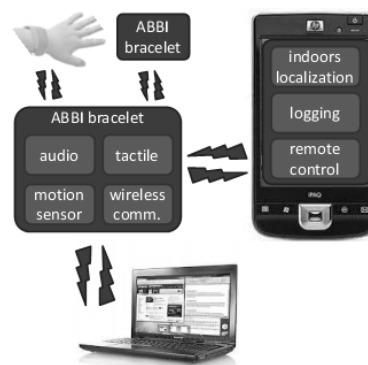
Figure 2. ABBI wireless smart station. The bracelet is communicating with a smart station (i.e. smartphone or computer) that allows changing parameters as the preferred sound and the volume. The station also stores data regarding the movement of the subjects.
