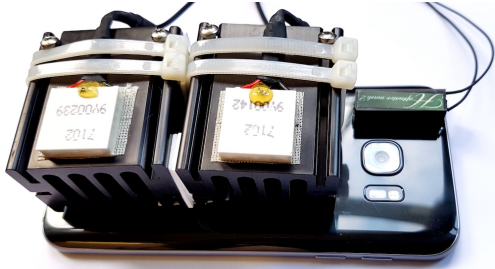
Figure 2: Device used for demonstration: Android phone with 2 x 2cm 2 Peltier devices and Haptuator Mk II on the back.
