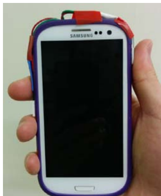
Figure 2: Experimental device: Samsung Galaxy S3 with 2 force-sensing resistors attached: one under the thumb and one under the middle finger.
