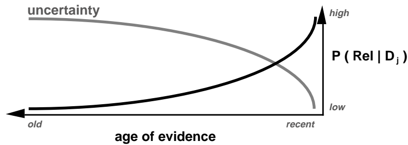
Figure 11: The inverse relationship between uncertainty and the object-conditional form of Ostensive Relevance.
