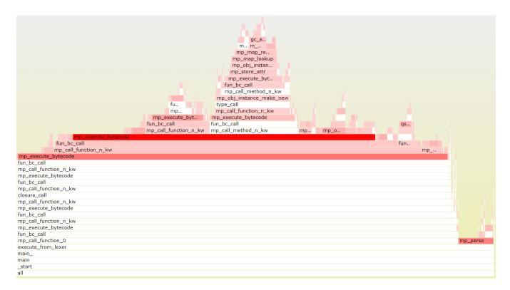
**Figure 8.** Differential Flame Graph (instructions retired) of purecap interpreter (after VM\_MAX\_STATE\_ON\_STACK adjustment) running pystone benchmark, relative to hybrid.
