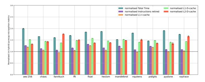
**Figure 9.** Performance of Python benchmarks running on the purecap interpreter with increased block size and maximum VM state size and a patched binary eliminating certain compiler inefficiencies, normalised to the hybrid interpreter performance.
