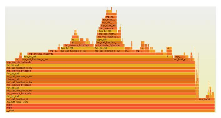
**Figure 4.** Flame graph (in terms of instructions retired) for hybrid version of MicroPython interpreter running pystone benchmark.
