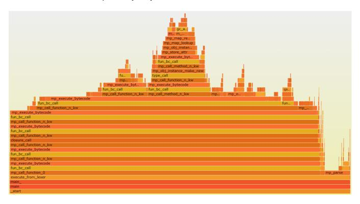
**Figure 7.** Flame Graph (instructions retired) of purecap interpreter (after VM\_MAX\_STATE\_ON\_STACK adjustment) running pystone benchmark.
