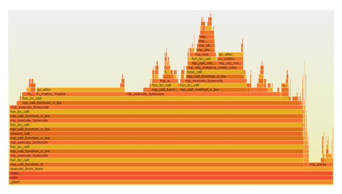
**Figure 5.** Flame graph (in terms of instructions retired) for purecap version of MicroPython interpreter running pystone benchmark—notice the large gc\_alloc horizontal bar.
