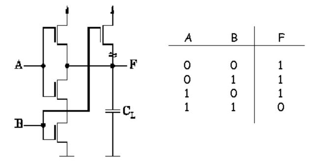
CMOS - NAND Gate - fault detection on: (A1, B1, A1, B0), (A1, B1, A0, B1) and (A1, B1, A0, B0).
