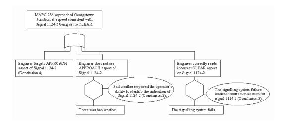
• Probabilistic inhibit gates.
