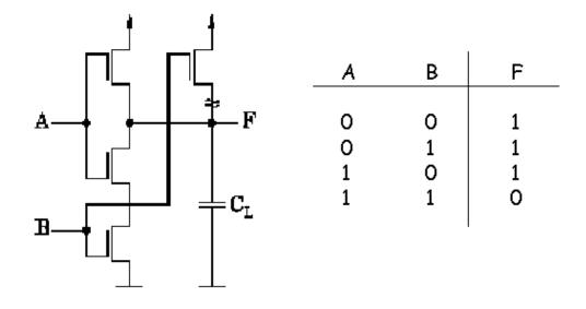
CMOS - NAND Gate - fault detection on: (A1, B1, A1, B0), (A1, B1, A0, B1) and (A1, B1, A0, B0).
