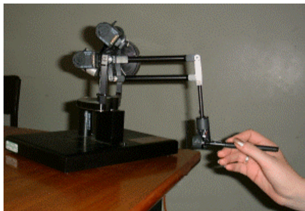
Figure 1: The Phantom 3D force feedback device from SensAble Technologies.
