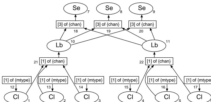
Fig. 1. Channel diagram of the load balancing example—clients are denoted Cl, servers Se and load balancers Lb.
