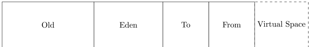
Figure 6.1: Parallel scavenge default heap layout
