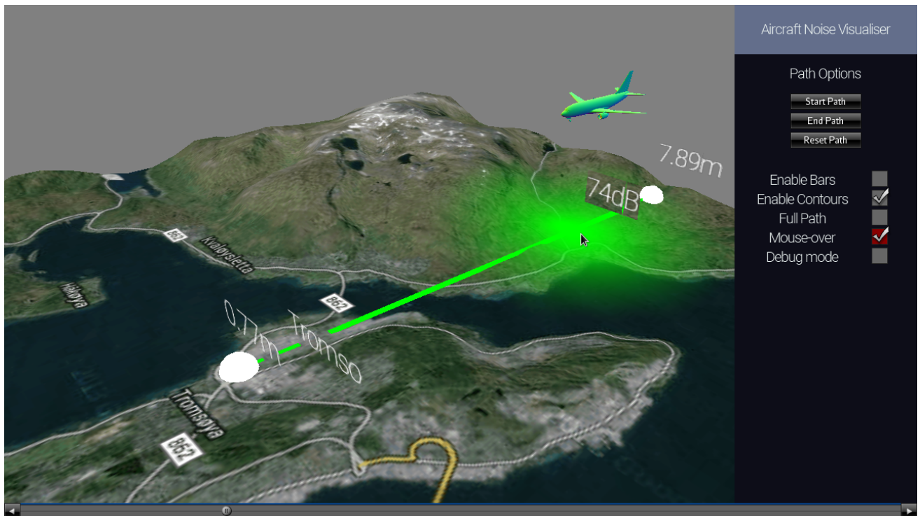
Figure 4.9: Aircraft landing at Tromsø airport. The green area depicts the noise levels on the ground. The user has used the mouse-over feature to measure the noise level at a specific point.
