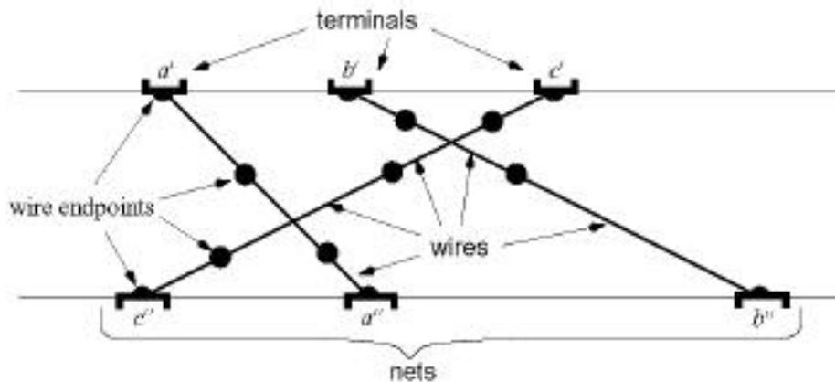
Figure 6: Two-dimensional Topological Model
