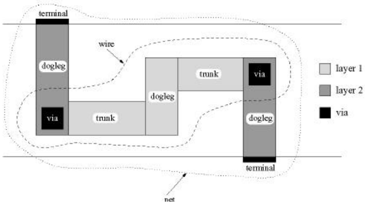
**Figure 4:** Channel Routing Definitions
