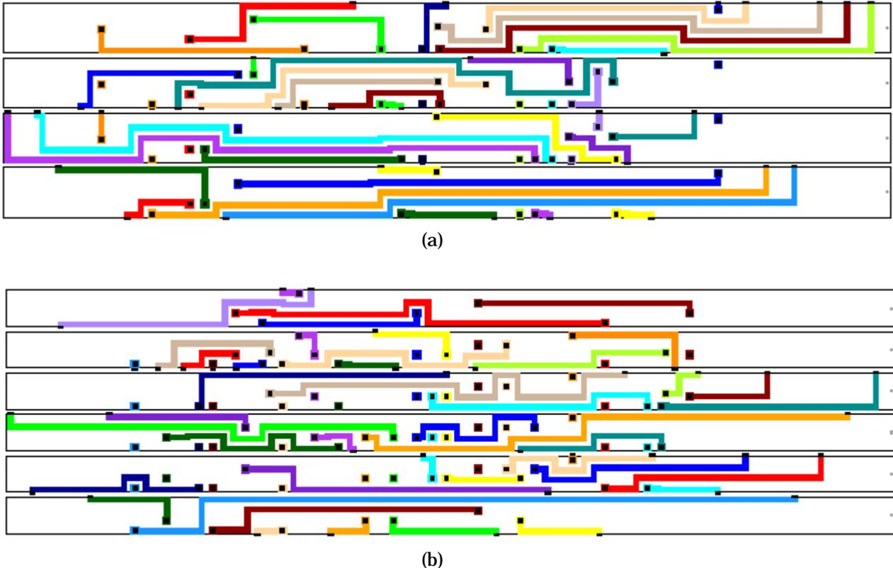
**Figure 15:** Complete routing example with 18 nets and congestion of 12. Figure (a) uses 4 layers, while (b) was given 6.
