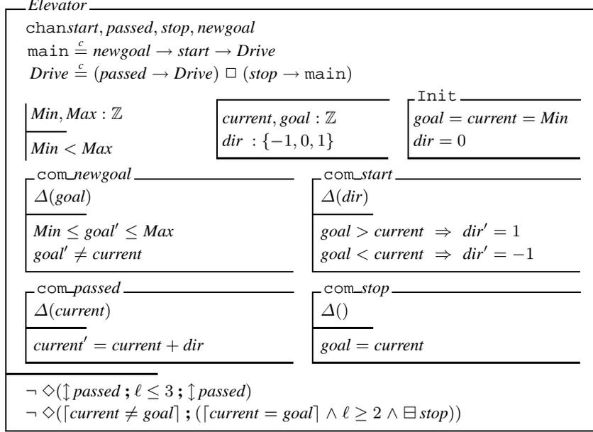
Fig. 2. Elevator specification
