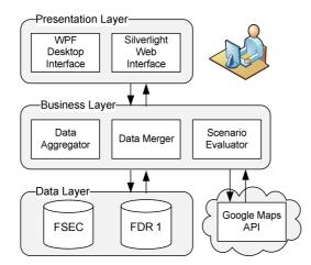
Figure 4: Data Flow and System Architecture of the Developed Prototype
