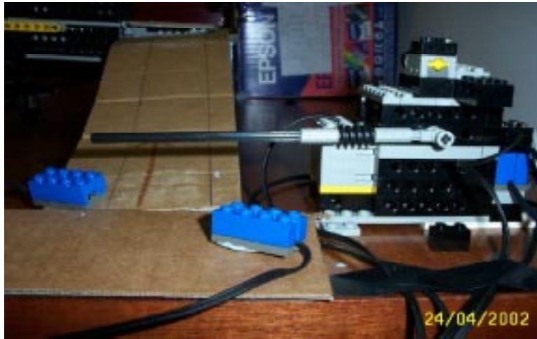
Figure 8: Barrier system with entry light sensors
