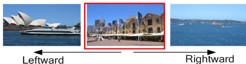
Fig. 1. Example of a tilt-based browsing UI (The red rectangle denotes the current view screen, referred as a cursor)
