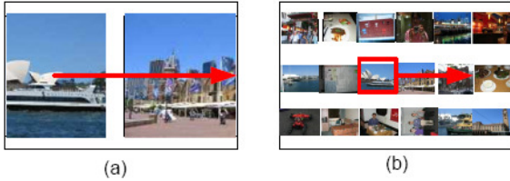
Fig. 9. Movement of a cursor (a) Local view: a cursor, the screen itself, moves leftward or rightward (b) Global view: a cursor mark (the red rectangle) moves over photos. The photos are scrolled only when the cursor moves out of them.
