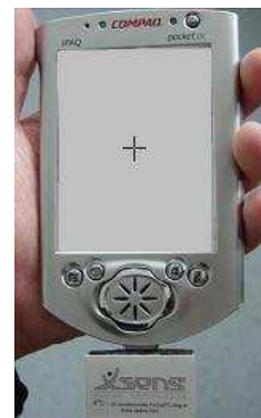
Figure 1. PDA with the Xsens P3C accelerometer attached to the serial port.
