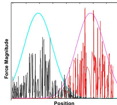
Figure 2(b). Magnitude of force vectors from two sources as the user moves left to right between their associated densities (the bell curves).
