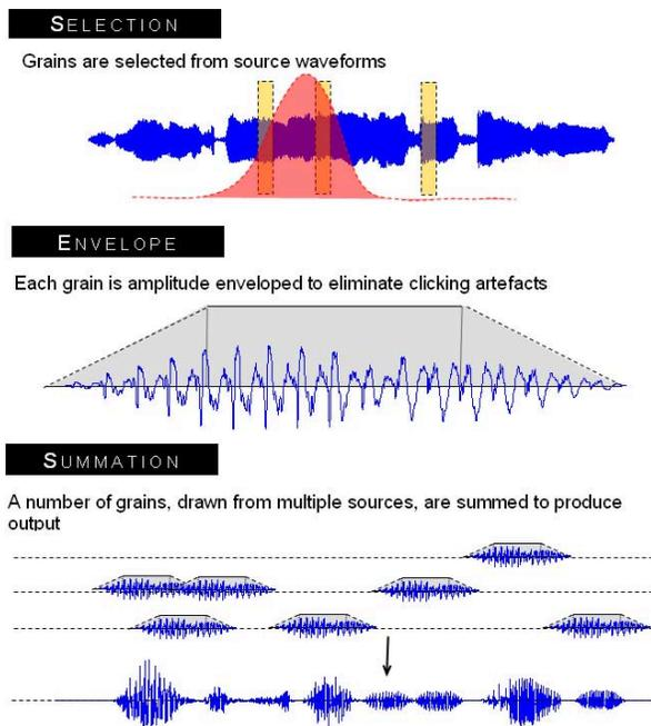
**Figure 1. A description of the granular synthesis process.**
