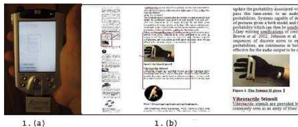
Figure 1: Pocket PC and accelerometer attached to serial port (1a). 3 screen shots of the document browser (1b) showing a red box moving rapidly over the picture (left), the user finding the picture and landing there (middle), and the zoomed-in picture (right).
