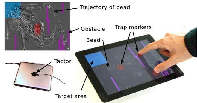
Figure 1: a) Running an experiment with the simulator on a tablet, with a user manipulating particles. b) Plots indicating user behaviour in one of the experiments.
