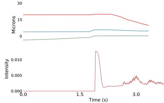
Figure 2: State evolution ( $x, y, z$ ) of a particle being trapped, then at 2.25s following as the user drags the trap. The lower plot shows the intensity of the vibrotactile response.
