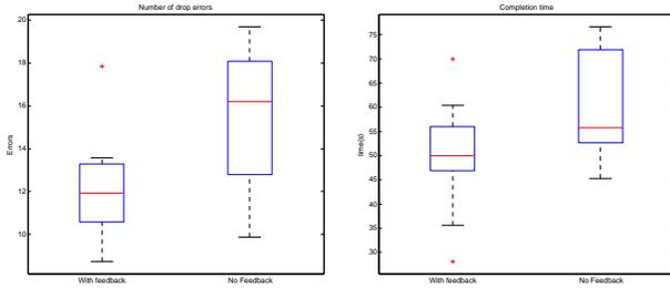
Figure 3: a) Box plots comparing error rates ( $N_e$ ) and time to completion ( $t_c$ ). With feedback,  $t_c$  was ( $\mu = 50.01s, \sigma = 10.91$ ), Without feedback  $t_c$  was ( $\mu = 60.04s, \sigma = 11.11$ ). With feedback  $N_e$  was ( $\mu = 12.14, \sigma = 2.34$ ), Without feedback  $N_e$  was ( $\mu = 15.39, \sigma = 3.45$ ).
