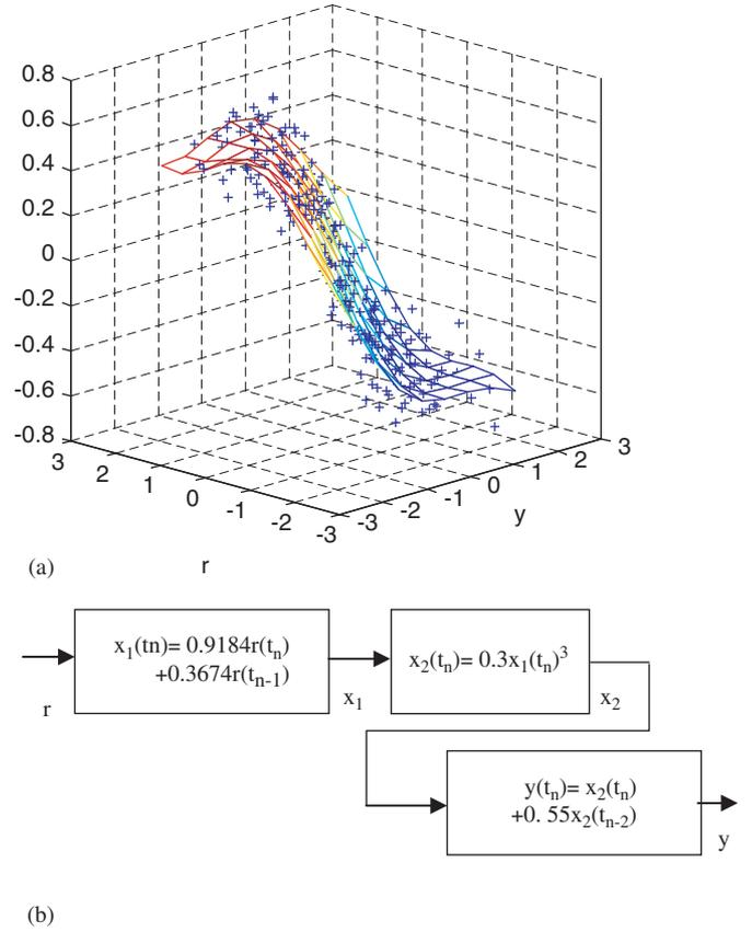
Fig. 1. (a) Measured data (+) and associated Gaussian Process model in Example (i) of Section 3.3, (b) Block diagram representation of system studied in Example (ii) of Section 3.3.
