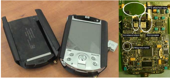
Figure 1. Left: MESH device alone and attached to an HP5550 Pocket PC. Right: The MESH circuit board showing the main components.
