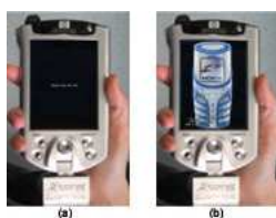
Figure 2: (a) The pocket PC requests that the user hold it. (b) The pocket PC has now measured the user's rest tremor.
