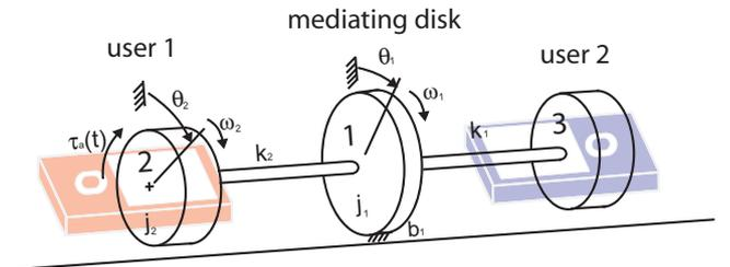
**Figure 3: Two users are connected with one disk to a mediating disk which has an oscillatory behaviour which is a function of the parameter settings and the input from each user.**
