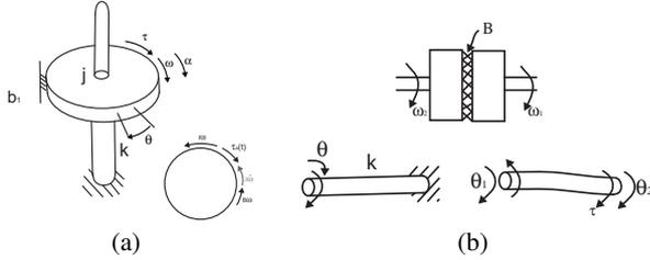
**Figure 2: (a) Rotational mechanical system conventions and a free-body diagram representing the forces present on the disk. (b) Rotational stiffness element with  $\Delta\theta = \theta_2 - \theta_1$ .**
