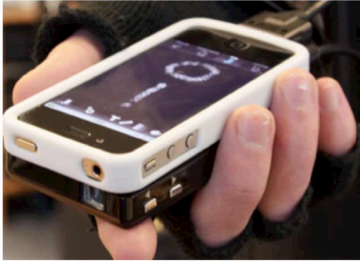
Figure 2. DigiGraff uses an iPhone 4 connected to a pico digital projector to create and display annotations.
