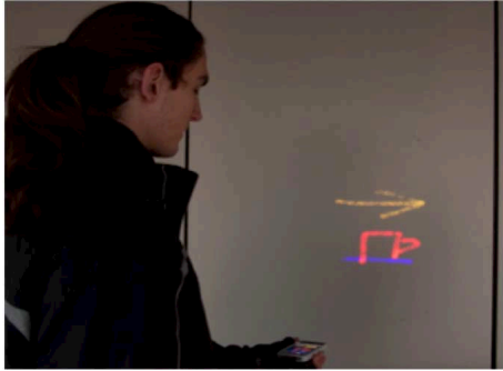
Figure 4. Users create their annotations by pointing the device at the location they wish to annotate and “spraying” it onto the environment. Similar to real graffiti, the annotation is geo-fixed and cannot be updated.
