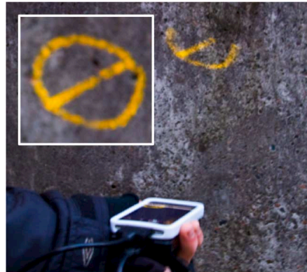
Figure 7. Using the iPhone's orientation sensors, the projector acts as a flashlight, progressively "illuminating" the fixed graffiti annotations as it is passed in front of them. Insert: the graffiti annotation once it has been fully uncovered.
