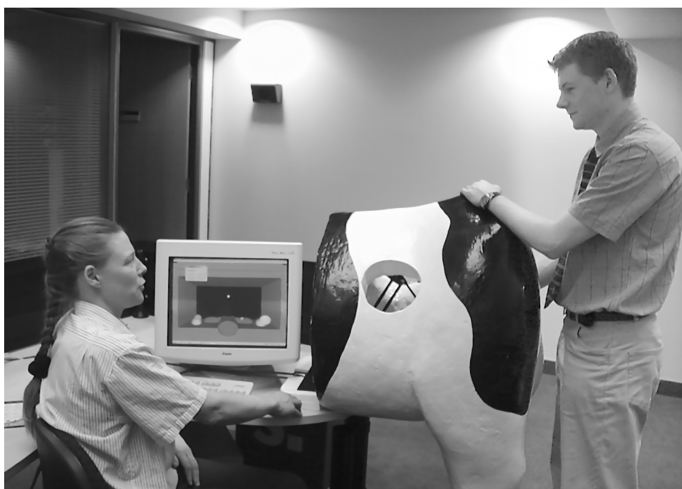
Figure 2: A simulator training session. The student palpates the virtual reproductive tract, receiving touch feedback from the PHANTOM haptic device positioned inside the fiberglass cow, while the instructor can follow progress on the computer screen and provide instructions
