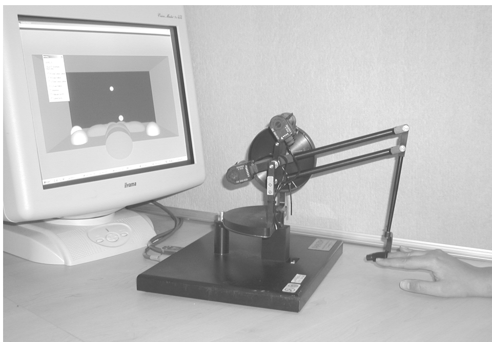
Figure 1: The PHANTOM force-feedback haptic device. The user places a finger in a thimble at the end of the mechanical arm and palpates virtual objects, in this case the bovine reproductive tract, depicted on the computer screen
