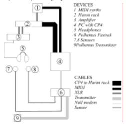
Figure 2: TouchMelody's hardware setup.
