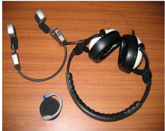
**Figure 1. The different headphone types used in the experiment. Bottom left is the single earpiece, top left are the bone conduction headphones and to the right are the Sennheiser headphones.**
