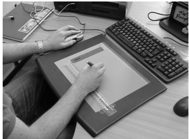
Figure 3. A user interacting with the prototype interface. Input is controlled via the graphics tablet with the dominant hand, while the non-dominant hand receives tactile feedback.
