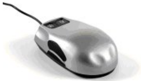
Figure 1a. VTPlayer mouse incorporating two tactile pin arrays.
