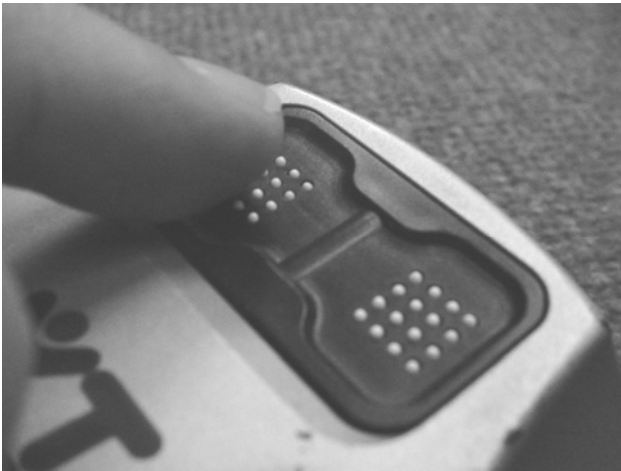
Figure 1b. Close up of the tactile pin arrays, two four-by-four matrices of individually controllable pins (shown with fingertip for scale).
